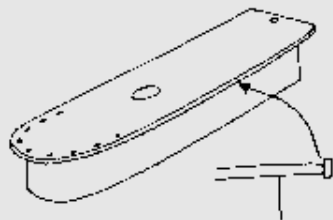
FIG. 12 – Adding the Cabin Top
